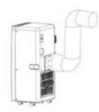
Slide the Hose Connector (Air Conditioner End) into the grooves.
