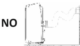
8. If you are not going to use the device for a long time, take the hose out of the window adapter and close it with the cover.
